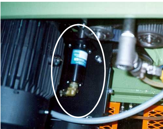
Figure 7 Resolver as mounted under Liner
